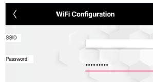
After the SSID and password are entered, the user can then send the WiFi settings to the wireless gateway module. If successful, the MODE LED (D, Figure 1) will be dark blue. If it failed, the MODE LED (D, Figure 1) will be red. Please try again.
